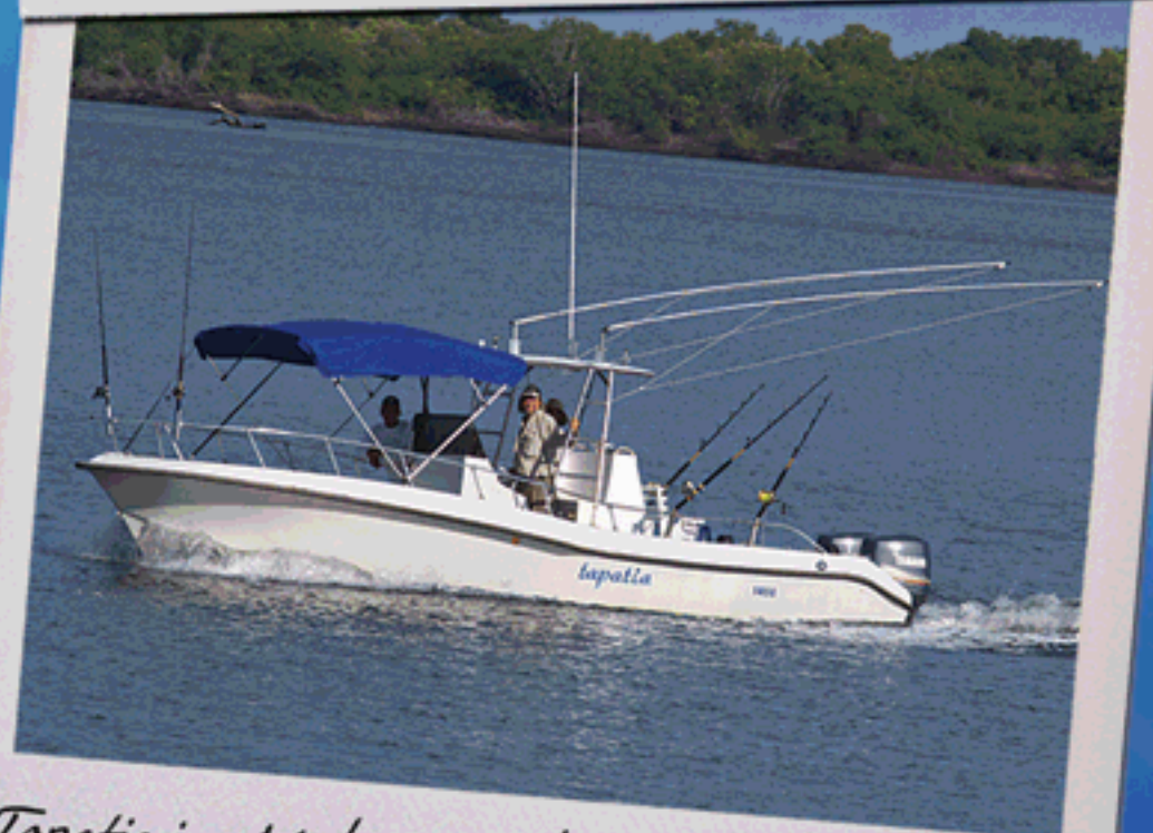
Tapatia is a Mako 28' fishing boat with two Yamaha 200 HP engines and has an 8 person capacity.
